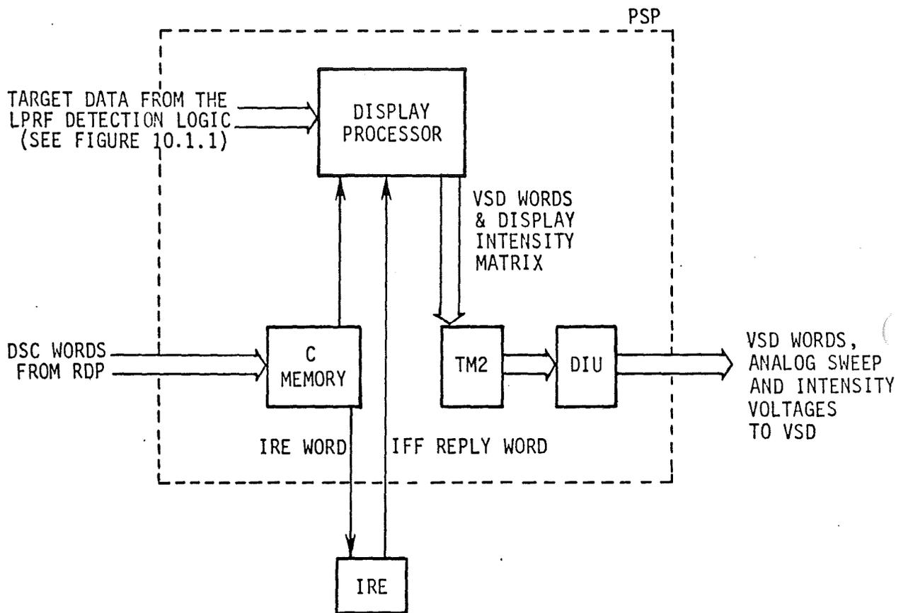
FIGURE 10.5.1 DATA FLOW BETWEEN THE PSP, RDP, IRE
