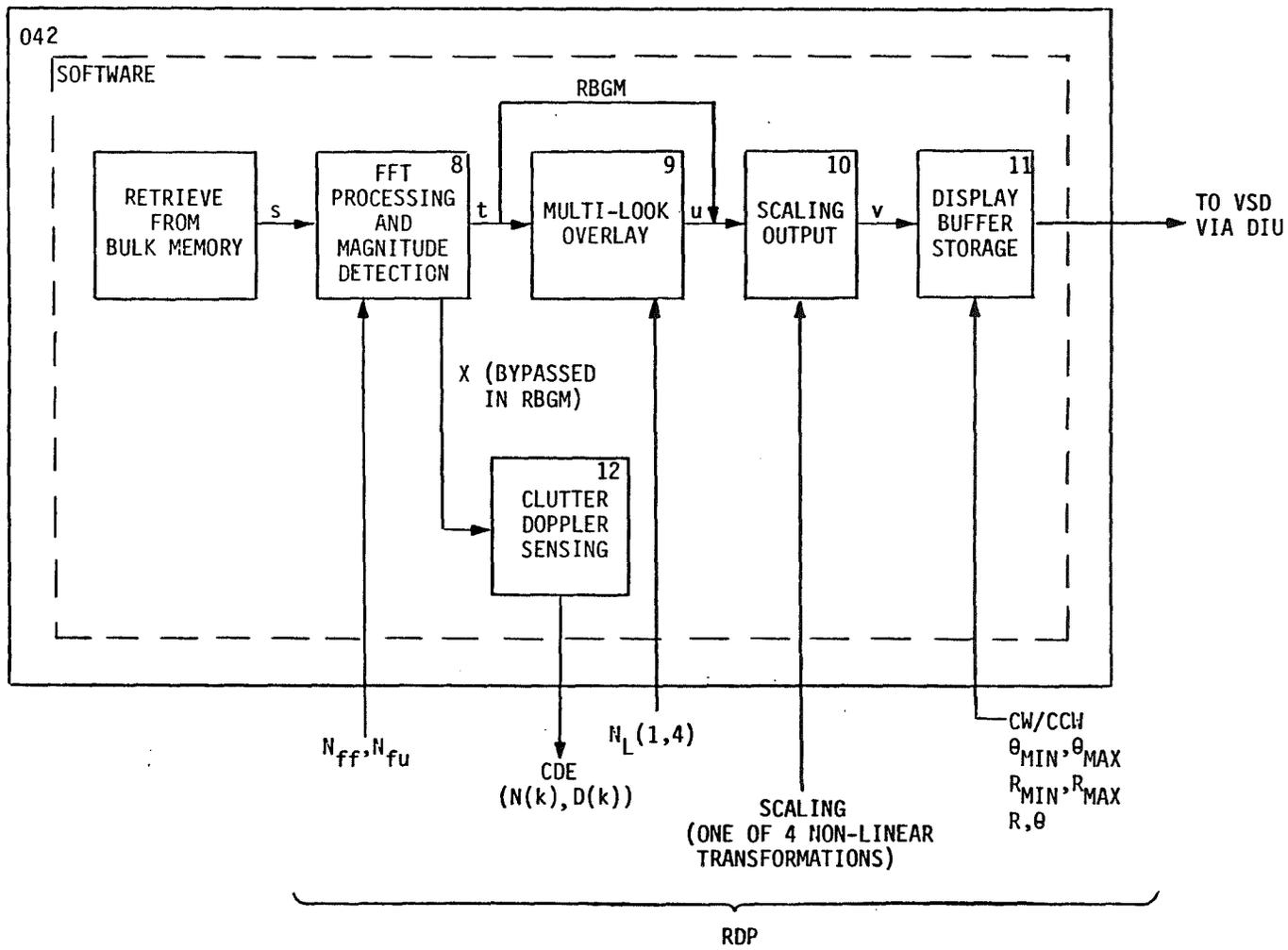
Figure 9.1b - DBS FFT AND POST PROCESSING
