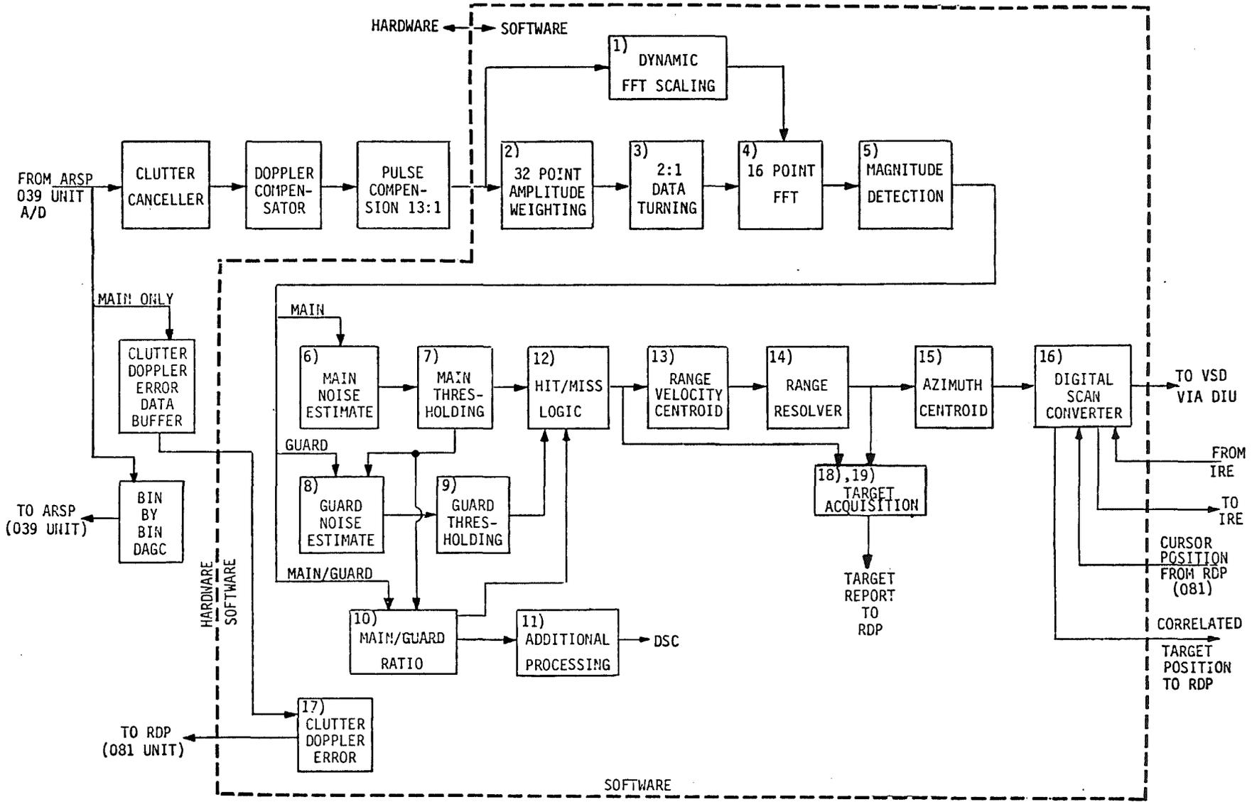
Figure 4.1 - F-15 SOFTWARE FUNCTION BLOCK DIAGRAM MPRF SEARCH
