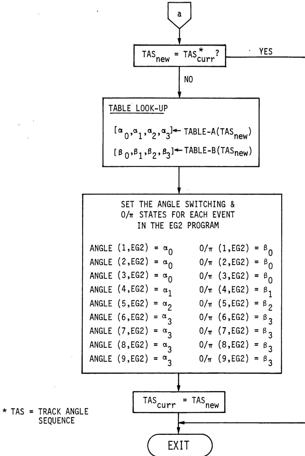
Figure 13.8 b - T&C TASK B - TRACK ANGLE SEQUENCE CHANGE
