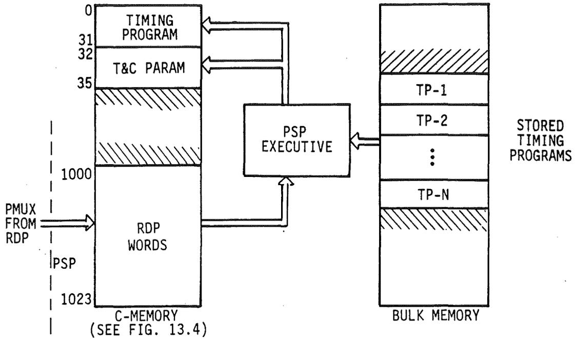
FIGURE 13.3.a - DATA FLOW FOR THE T&C FUNCTION - HPRF RAM STT MODE
