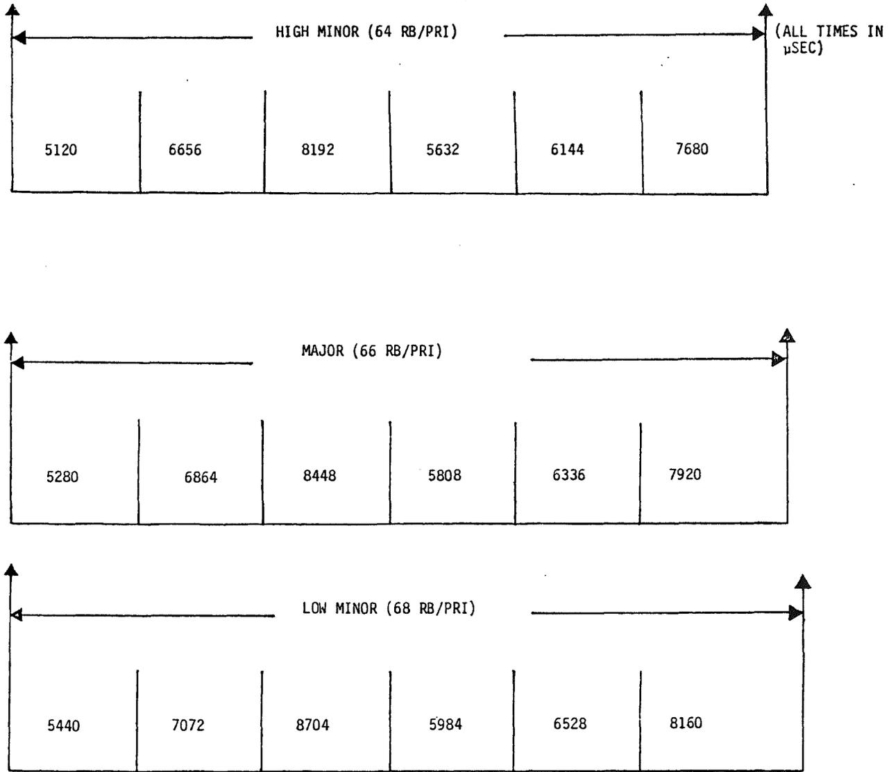
FIGURE 11.3 - RAM SCAN AND SPOTLIGHT I TIMING (64 DATA PULSES)
