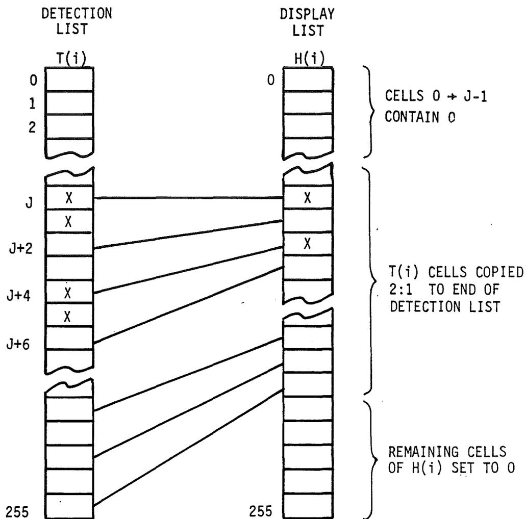
FIGURE 10.4.1 1X RANGE DISPLAY LIST PROCESSING
