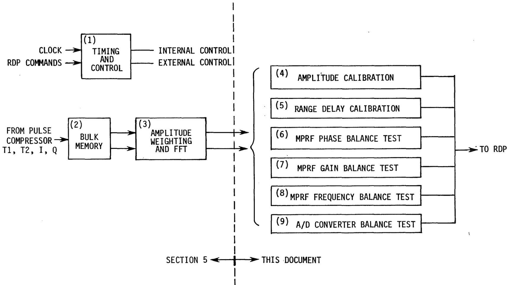
FIGURE 15.1 MPRF BIT CALIBRATION AND TEST DIAGRAM
