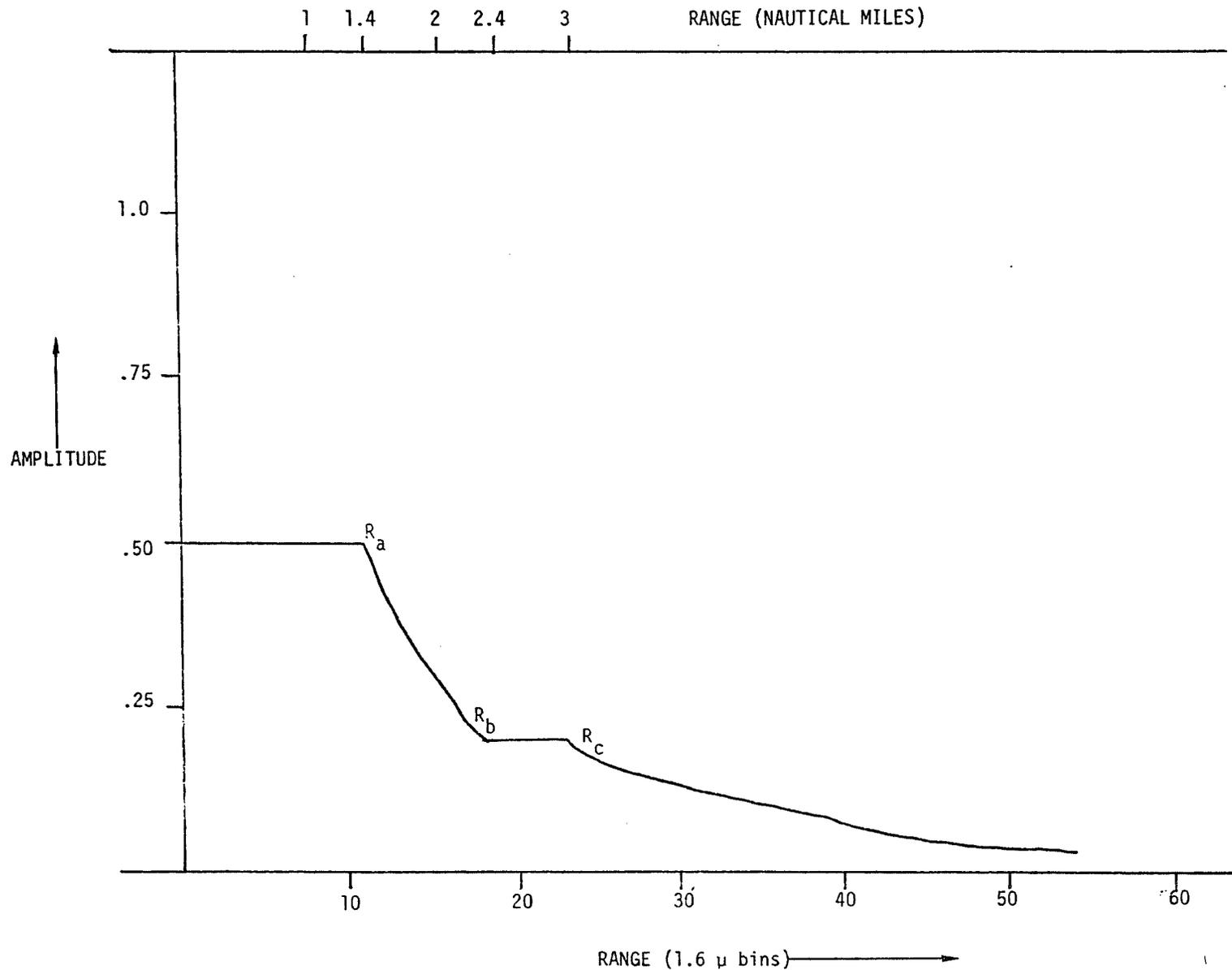
FIGURE 4.7 - RANGE VARIABLE THRESHOLD (RVT)
