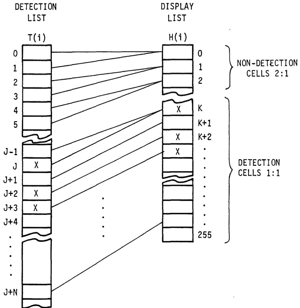
FIGURE 10.4.2 4X RANGE DISPLAY PROCESSING
