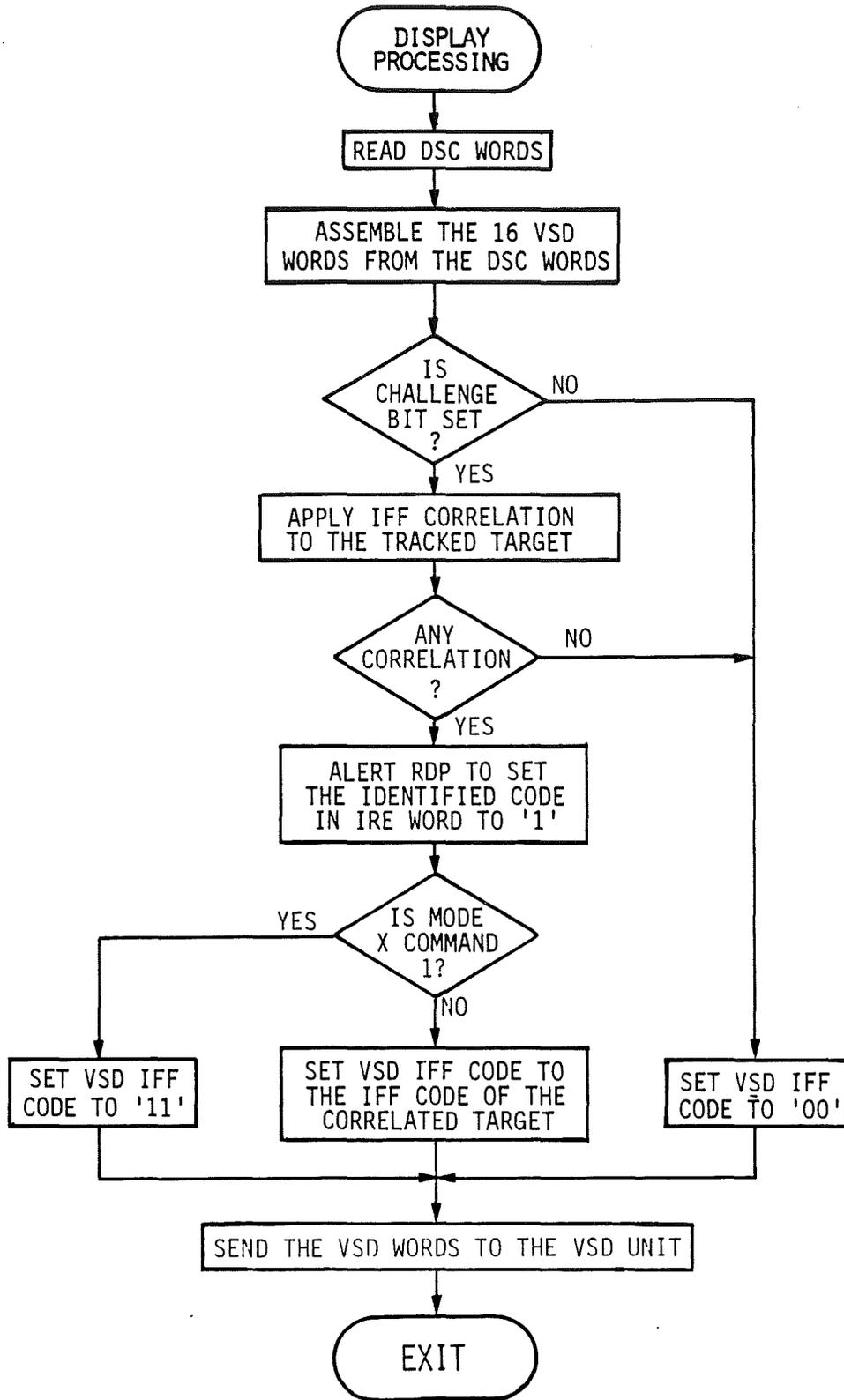
Figure 3.6.2 - HPRF TRACK DISPLAY PROCESSING
