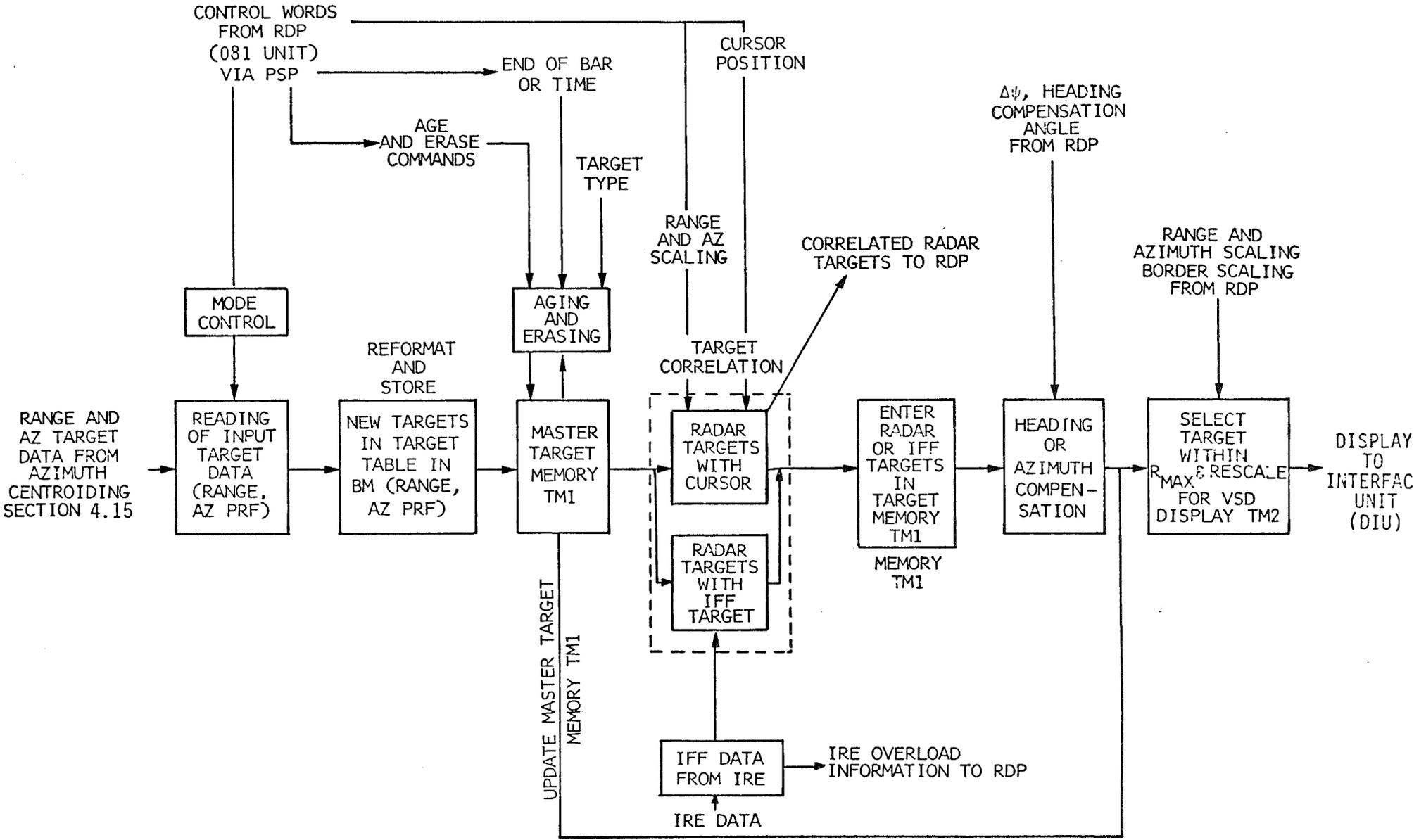
FIGURE 4-15 SYSTEM SCAN CONVERTED FUNCTION DIAGRAM FOR MRPE SEARCH ACC I AND ACC II
