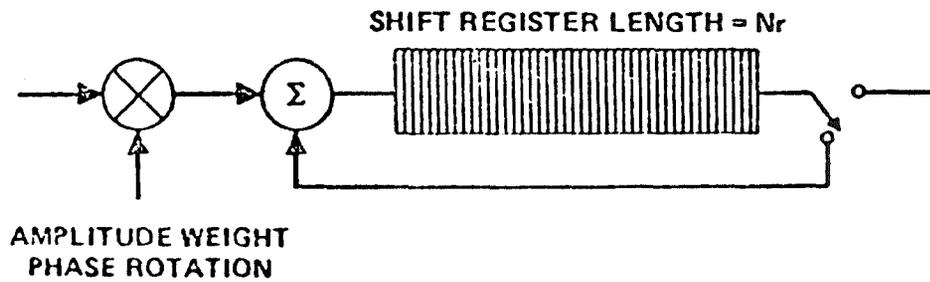
Figure 9.4.1 - PRESUM FILTERING ALGORITHM
