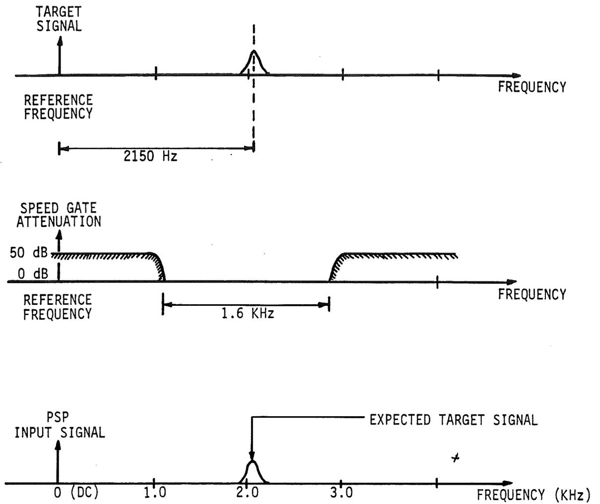
Figure 13.2 - TRACKED TARGET SIGNAL AND THE SPEED GATE
