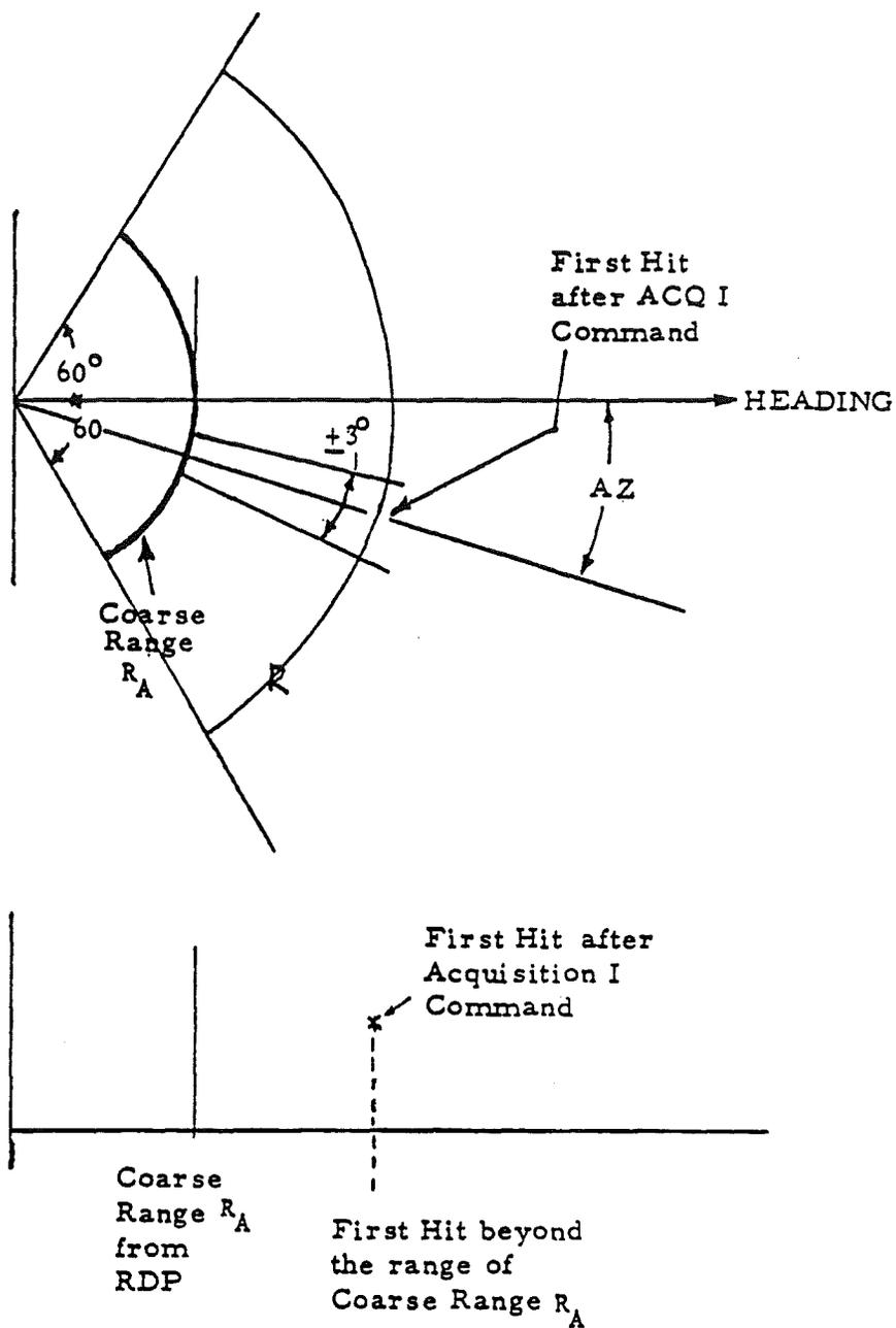
Figure 4.18.2 - MPRF ACQ I TARGET ACQUISITION
