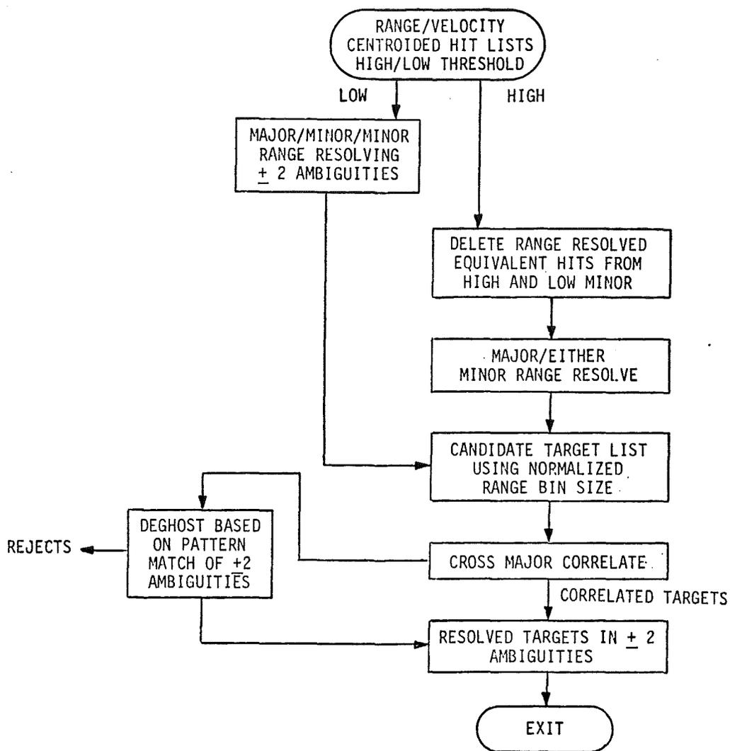
Figure 11.13.1 - RANGE RESOLUTION PROCESSING
