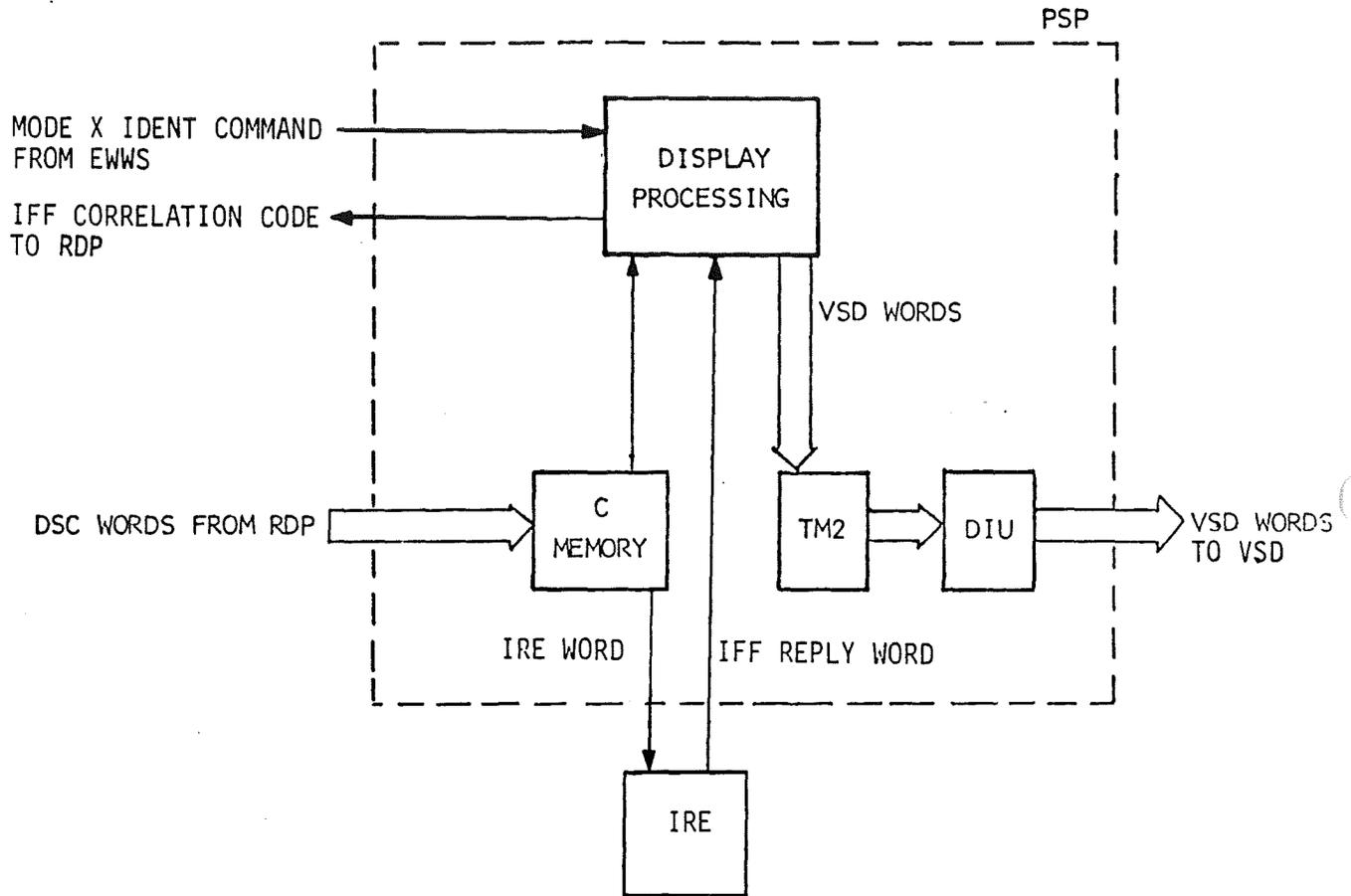
Figure 3.6.1 - DATA FLOW BETWEEN THE PSP, RDP, IRE AND THE VSD UNIT DURING DISPLAY PROCESSING
