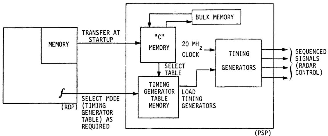
Figure 1.1.1 - TIMING GENERATOR SCHEME
