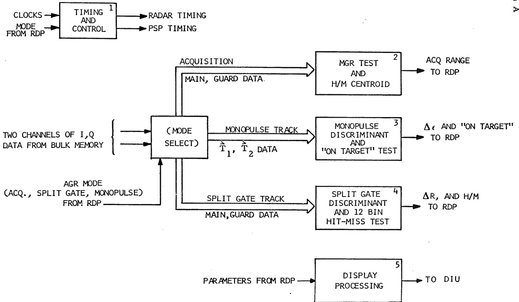
Figure 8.1 Air-to-Ground Ranging Modes Processing
