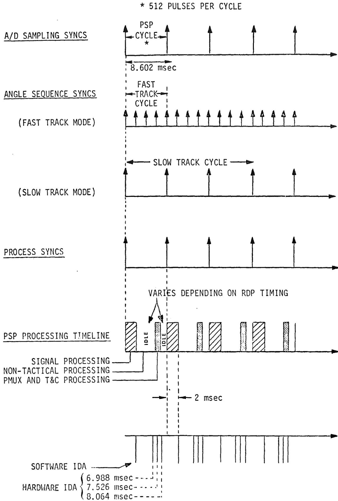
Figure 3.1.2 - HPRF TRACK TIMING FUNCTIONS
