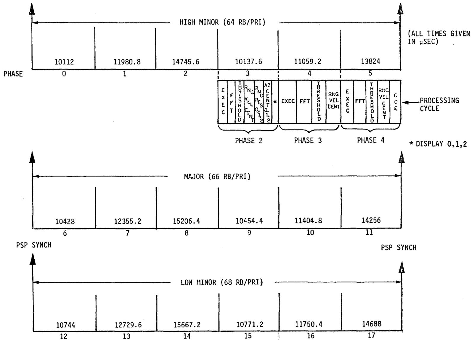
FIGURE 11.2 - RAM SCAN AND SPOTLIGHT I TIMING (128 DATA PULSES)
