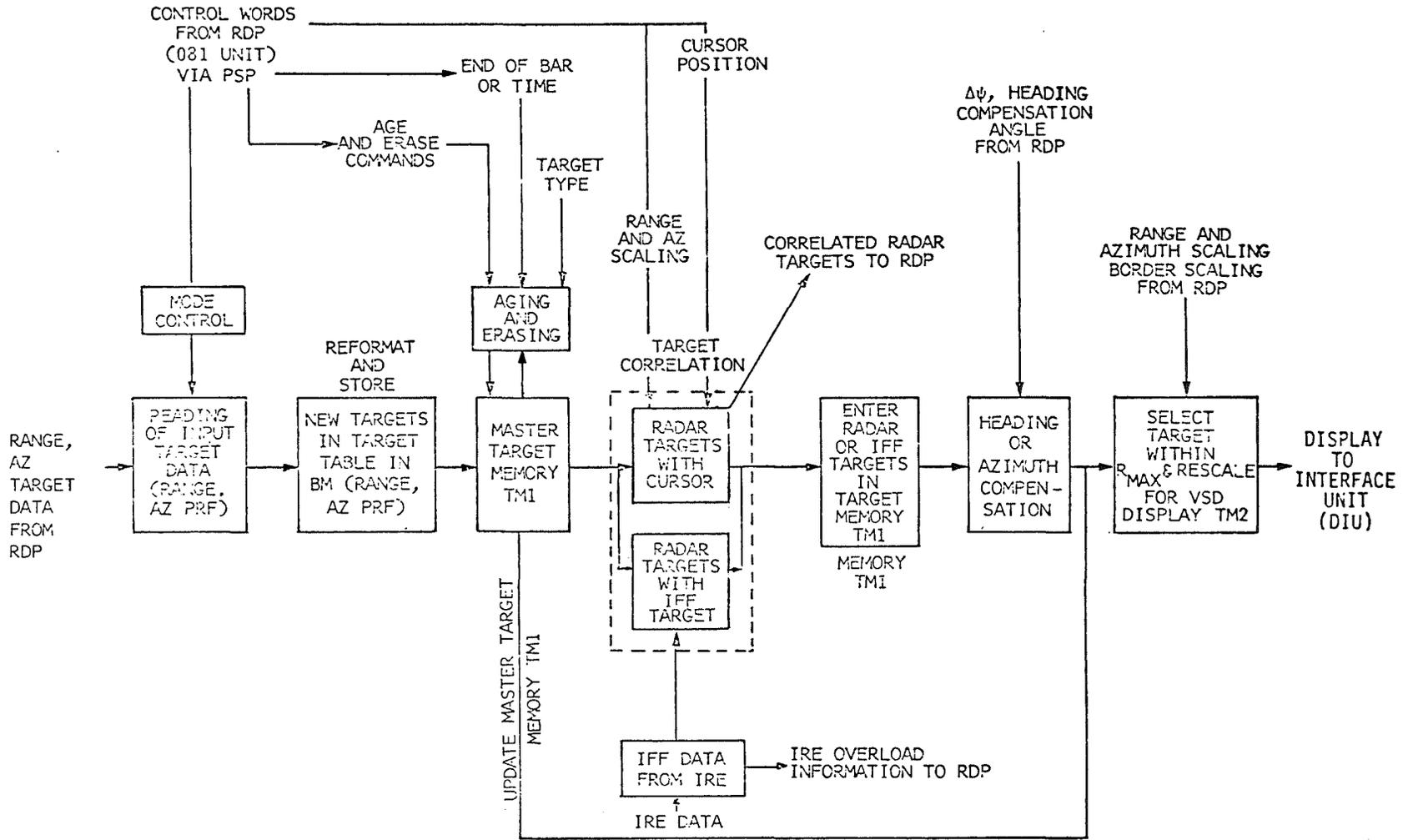
Figure 5.6.3 - DIGITAL SCAN CONVERTER FUNCTION DIAGRAM
