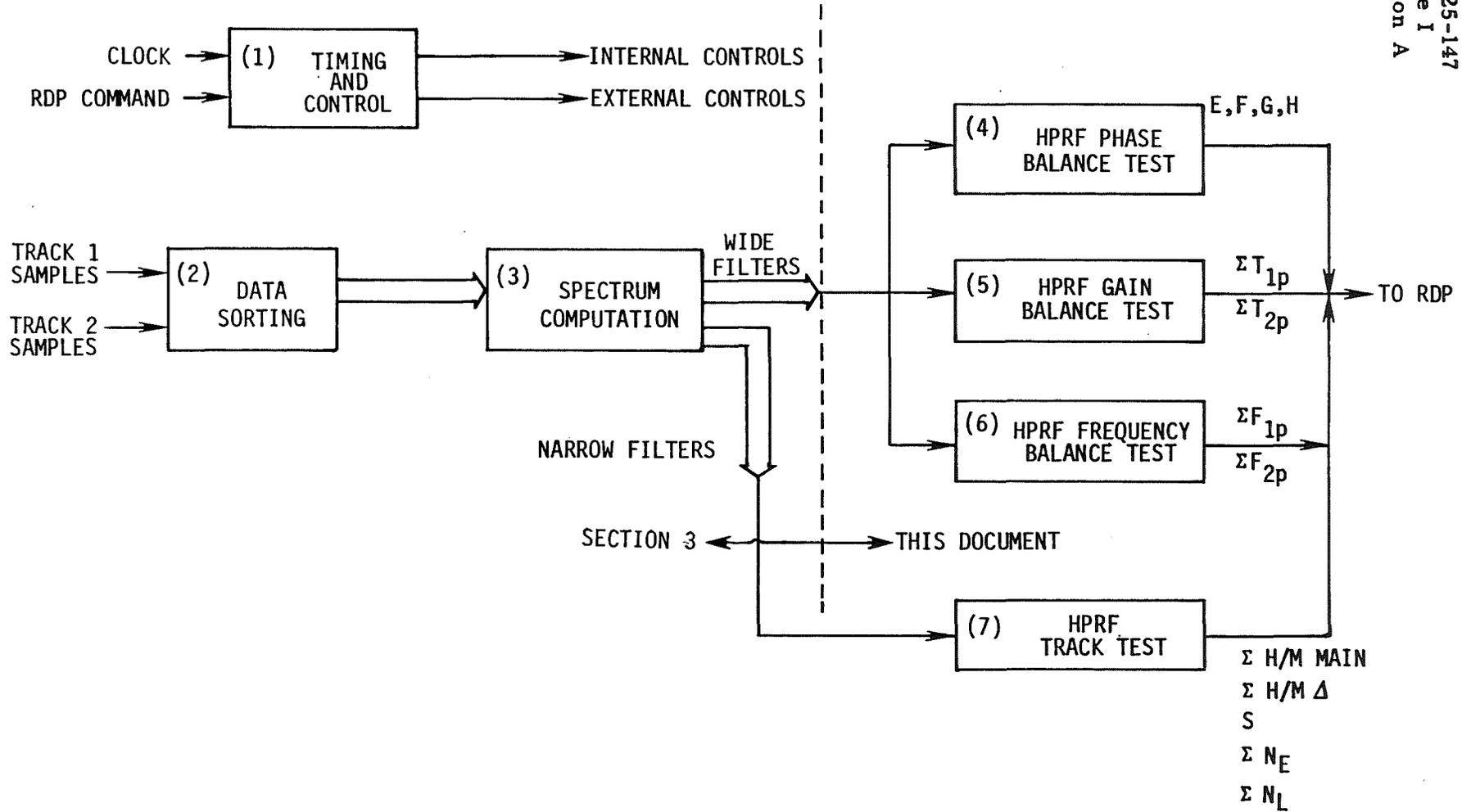
FIGURE 14.1. HPRF BIT TEST DIAGRAM
