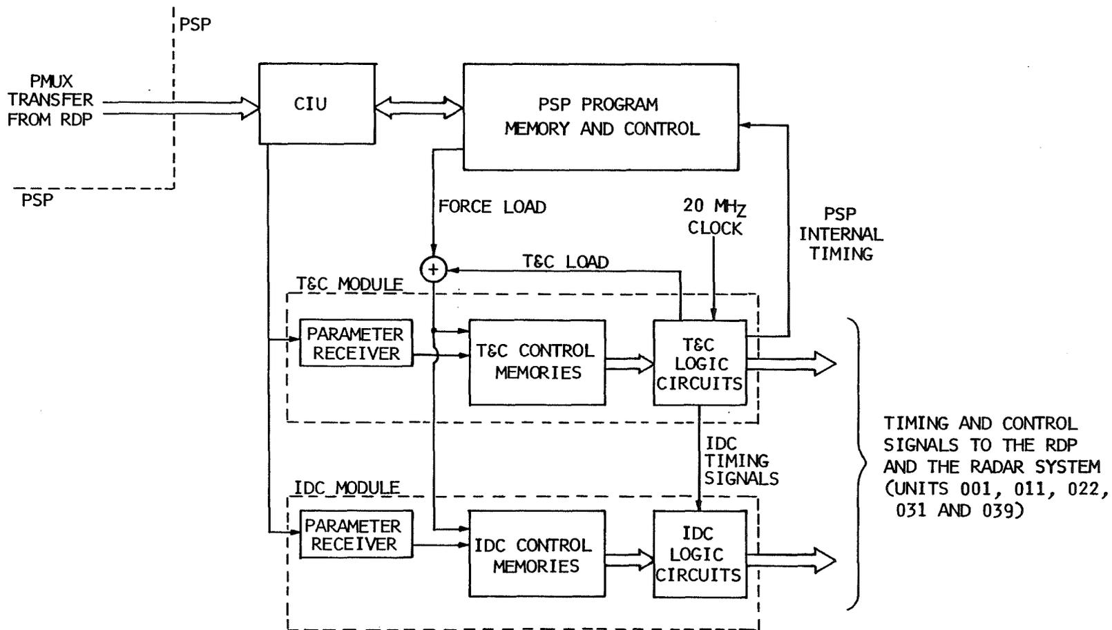
FIGURE 10.1.1 GENERALIZED SCHEMATIC SHOWING THE INTERACTION BETWEEN THE T&C/IDC MODULES, THE PSP MEMORY & CONTROL, THE CIU AND THE RDP.
