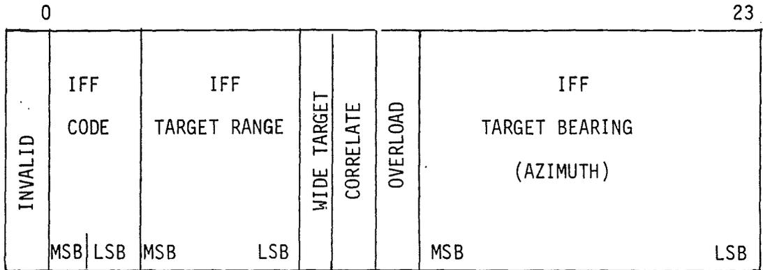
FIGURE 4.16.3 IFF REPLY WORD FROM IRE BUFFER
