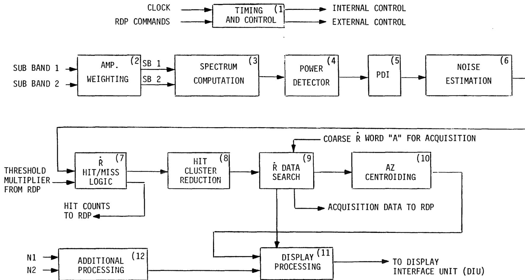
Figure 2.1 - HPRF  $\dot{R}$  SEARCH AND ACQUISITION FUNCTION DIAGRAM
