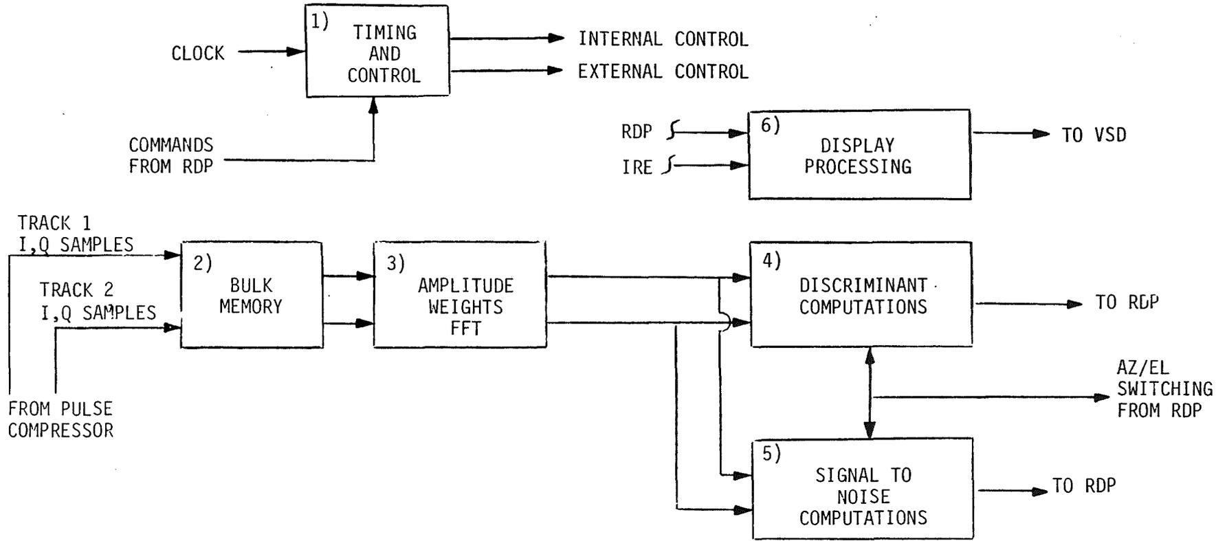
Figure 5.1 - MPRF TRACK PROCESSING
