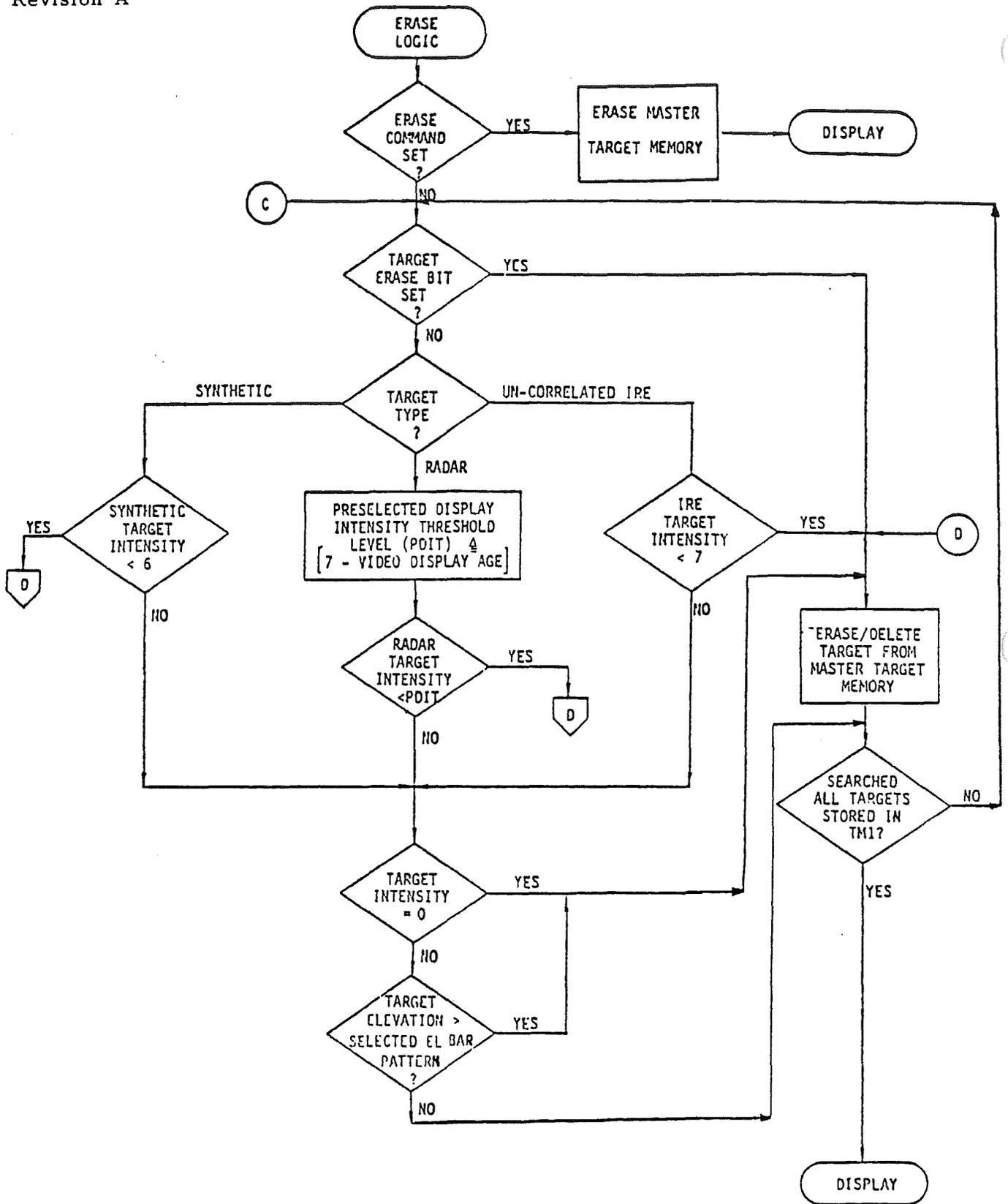
Figure 4.16.9 - TARGET/TARGET MEMORY ERASE LOGIC
