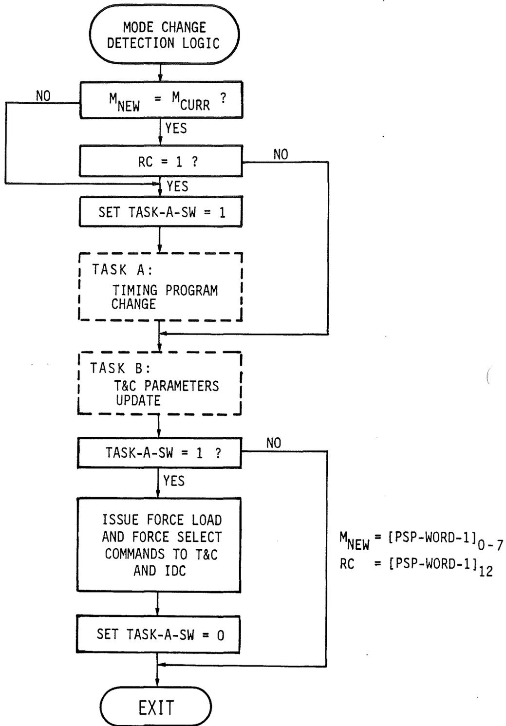
FIGURE 13.5 - MODE CHANGE DETECTION LOGIC
