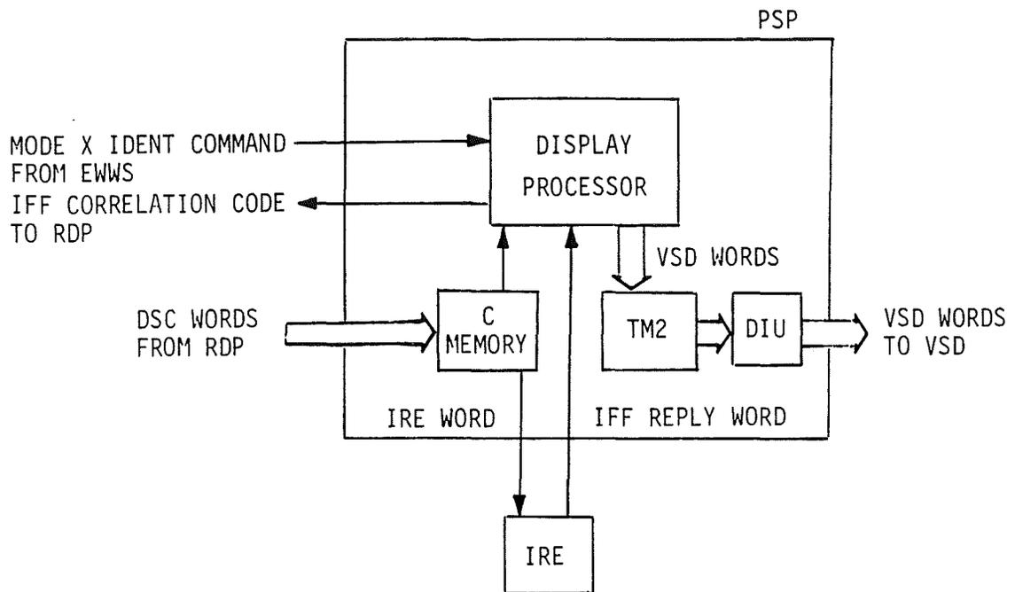
Figure 13.10 - DATA FLOW BETWEEN THE PSP, RDP,
