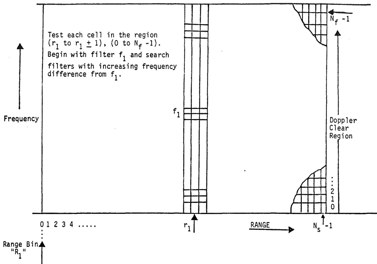
FIGURE 12.5.1 - RANGE/DOPPLER CELLS TESTED FOR HIT/MISS
