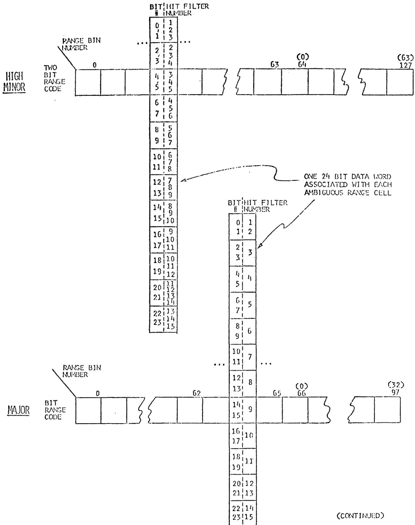
Figure 4.14.3 - TARGET HIT FILTER NUMBER ASSIGNMENTS IN RANGE DATA WORDS
