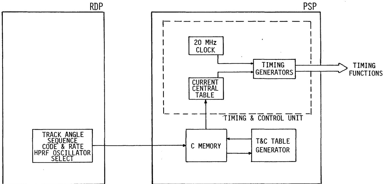
Figure 3.1.3 - INTERFACE BETWEEN THE RDP, PSP AND THE T&C MODULE
