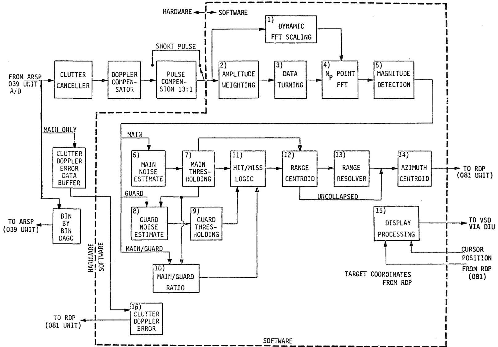
Figure 11.1 - RAM MPRF SEARCH SOFTWARE FUNCTIONAL BLOCK DIAGRAM MPRF SEARCH
