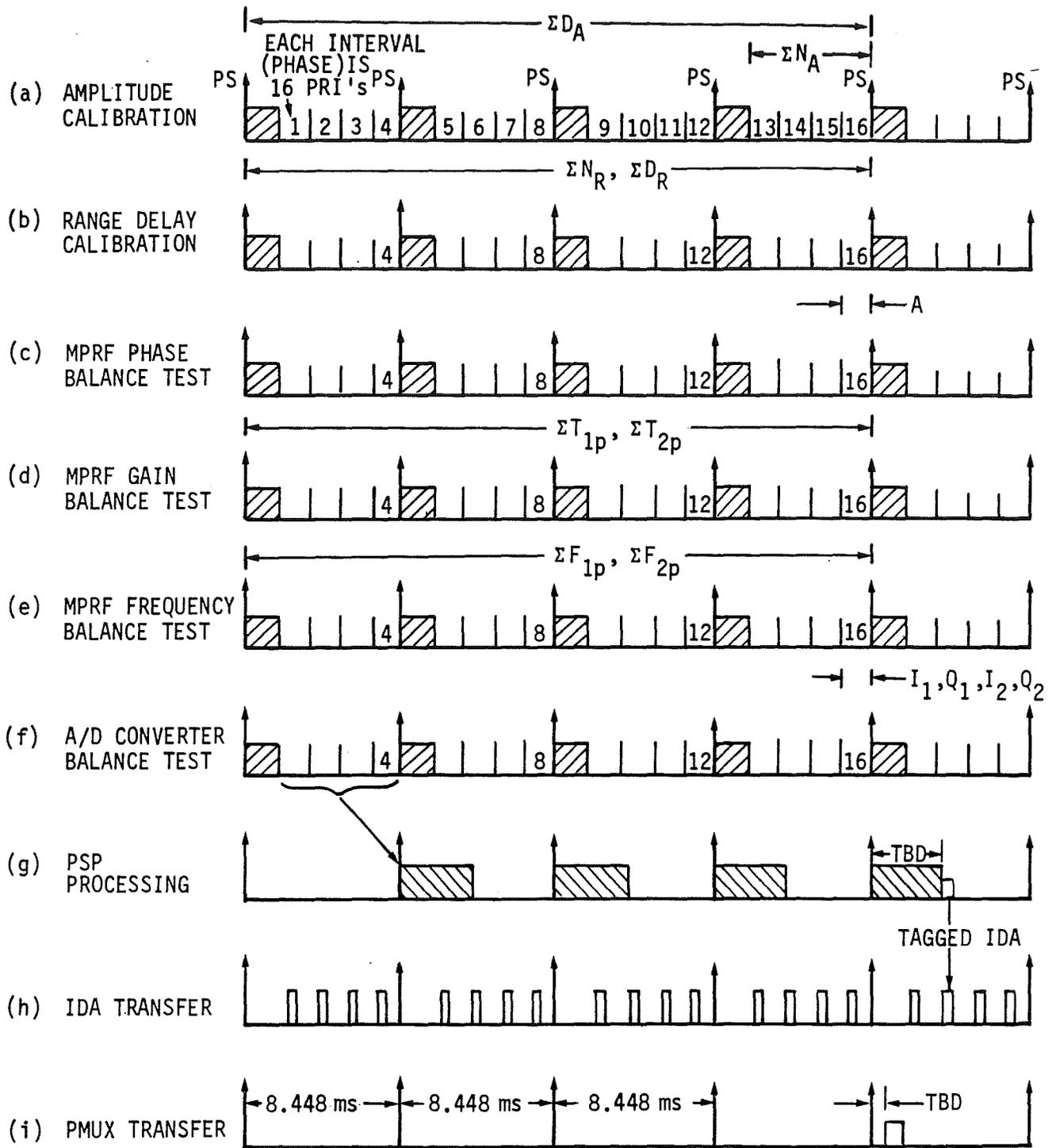
FIGURE 15.1.1. MPRF BIT CALIBRATION AND TEST MODE
