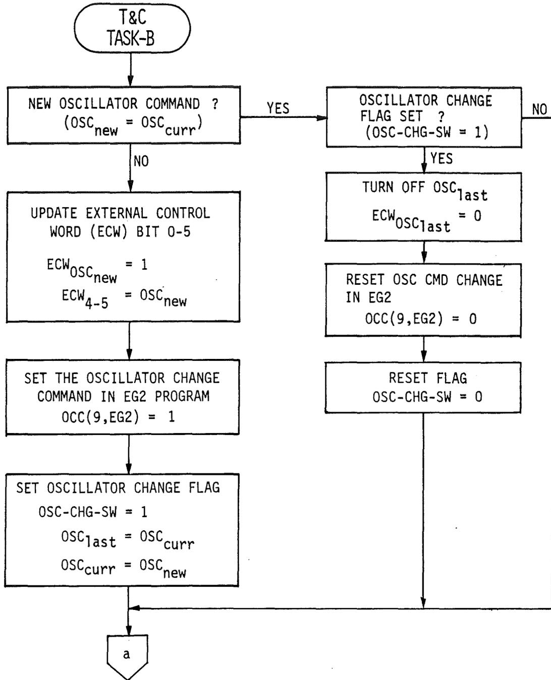
Figure 13.8 a - T&C TASK B - OSCILLATOR SELECTION CHANGE
