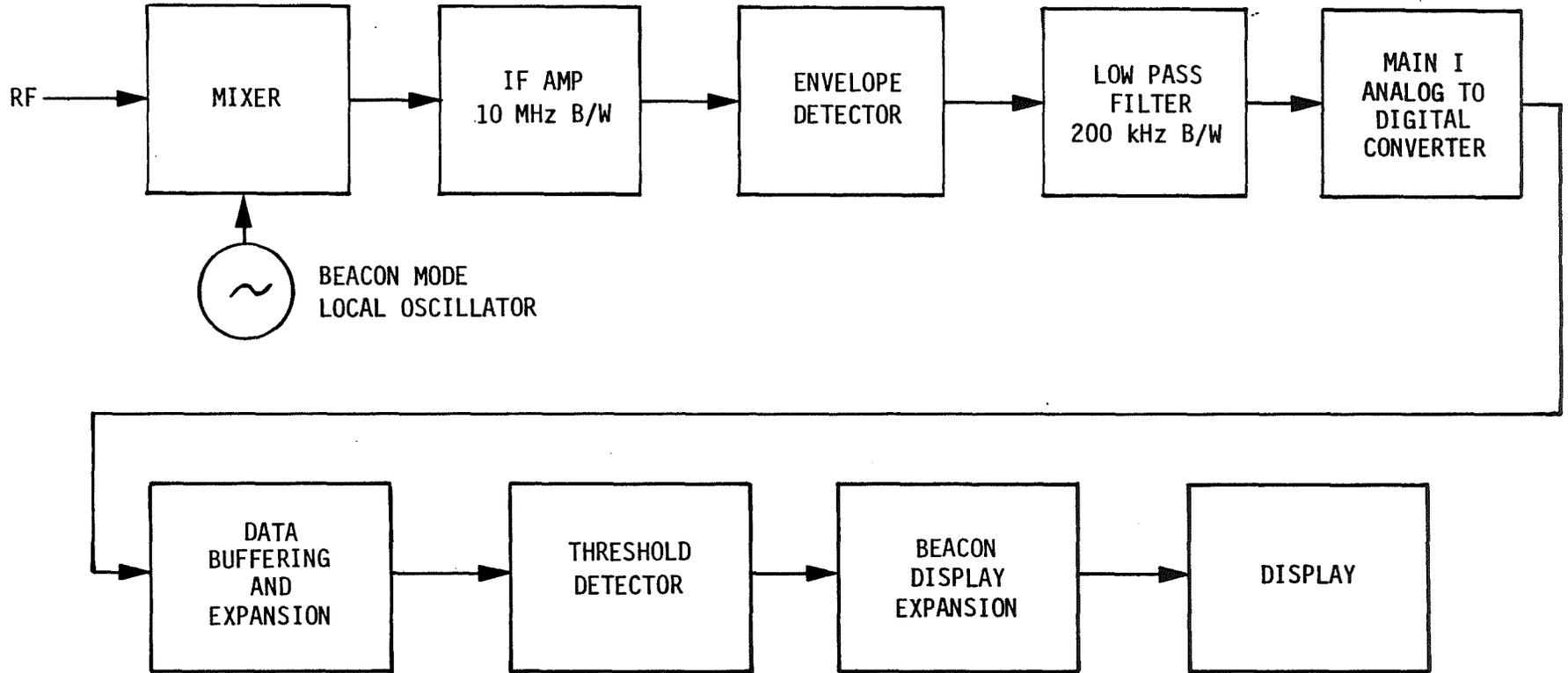
FIGURE 10.1. BEACON MODE - FUNCTIONAL DIAGRAM
