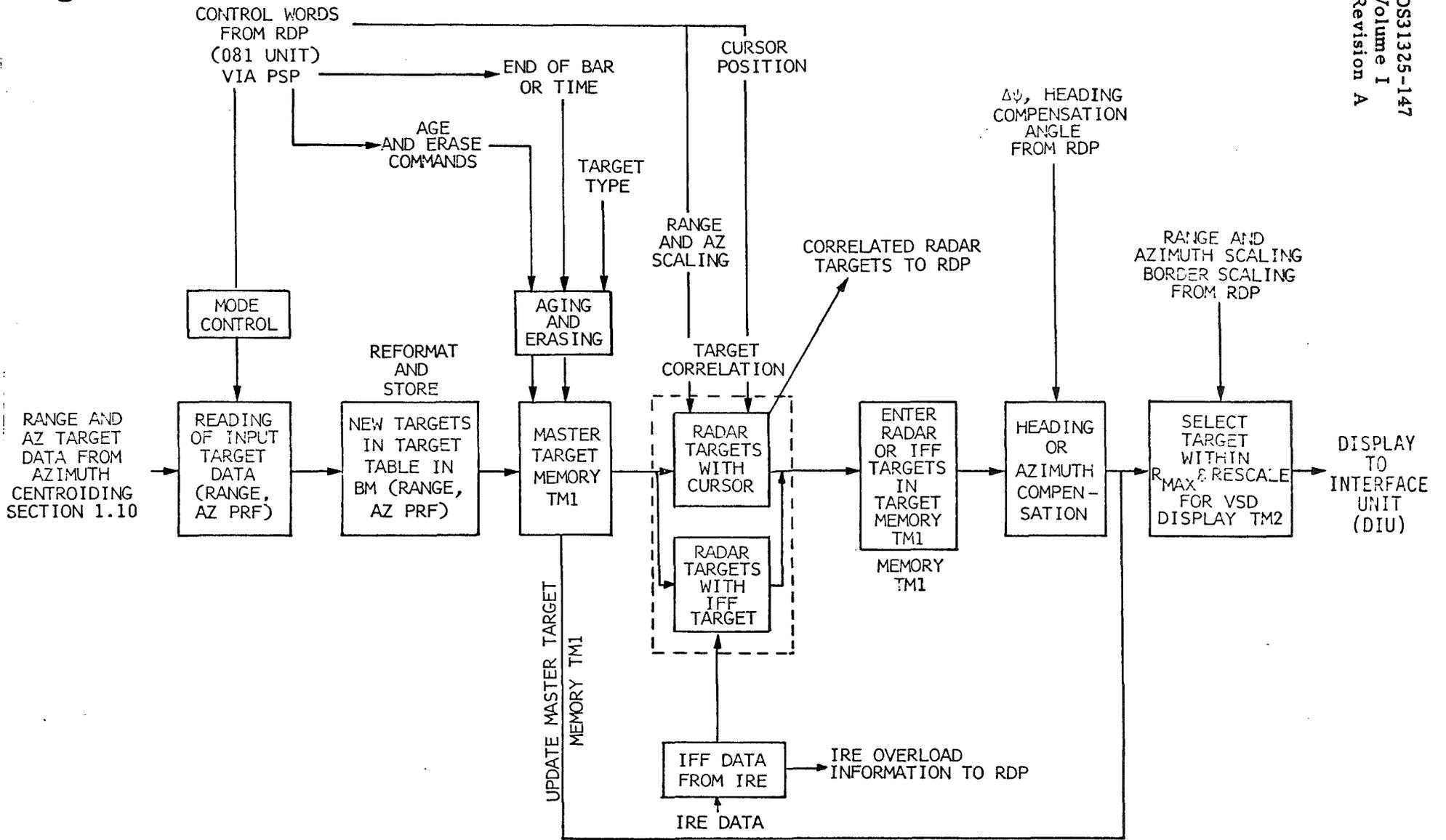
FIGURE 1.11.2 - DIGITAL SCAN CONVERT FUNCTION DIAGRAM HPRF RWS SEARCH
