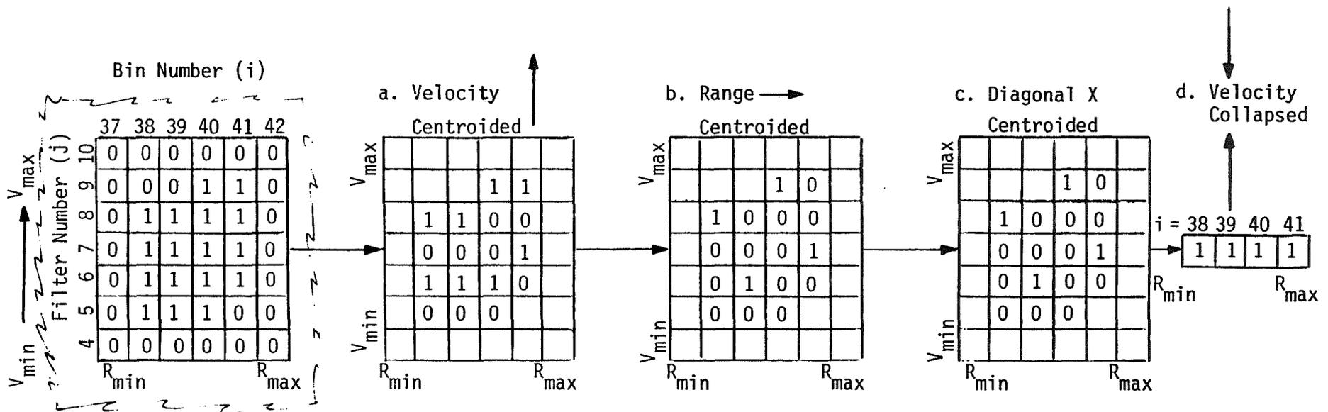
Figure 11.11.3 - EXAMPLE OF CENTROIDDING TECHNIQUE
