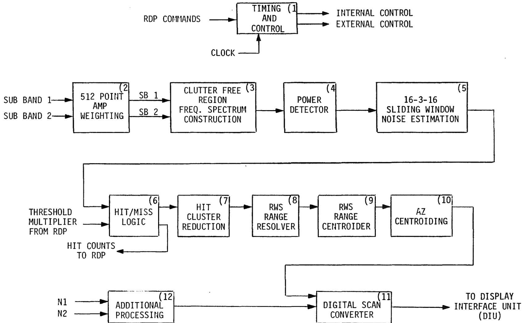
Figure 1.1 - RWS FUNCTION DIAGRAM
